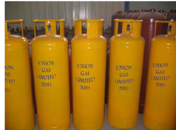
Ammonia refrigerant cylinders
